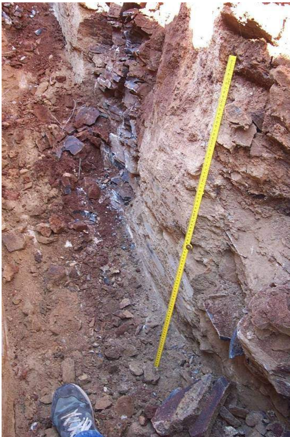
Figure 25 From 1 to 2 metres deep in the backhoe pit showing the edge of one basalt pillar flanked by two basalt pillars that have been broken in half.
