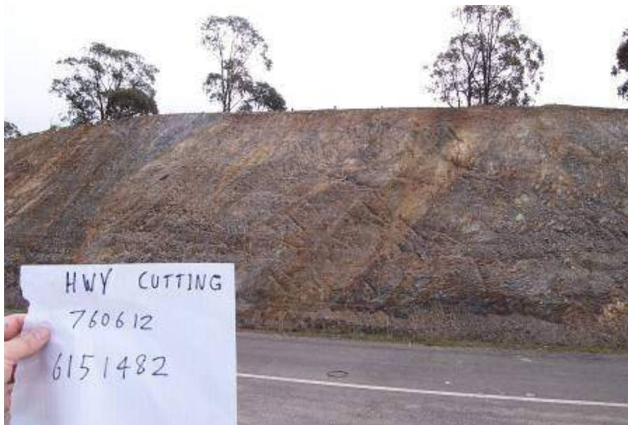
Figure 10 A highway cutting north of Marian Vale clearly shows the near vertical layering of rock in the area along with a near non-existent soil profile also common in the area. This site has been classified by NSW Geological Survey as Warbisco Shale. It is presented here because it is a good example of structure and weathering similar to that that cannot be observed under Marian Vale.
