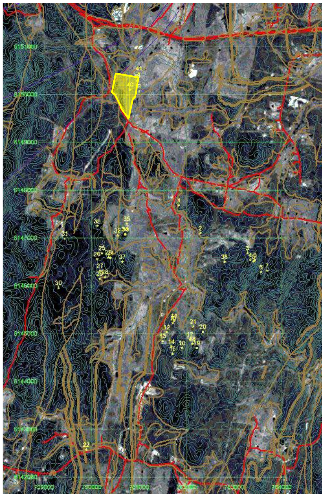
Figure 14 An overview of rock sample locations (in AGD66 coordinates), and NSW Geological Survey boundaries, contours roads and landsat (NSW Geol. surv. , 2003)
