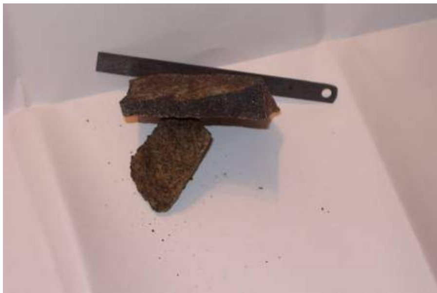
Figure 2 Basalt (hard durable fine grained rock – ‘blue metal’) and Gabbro (weathered coarse grained rock) from sample site 36. No gabbro was evident at the surface as it has been weathered away. This sample was collected from 2m metres down in the backhoe pit.
