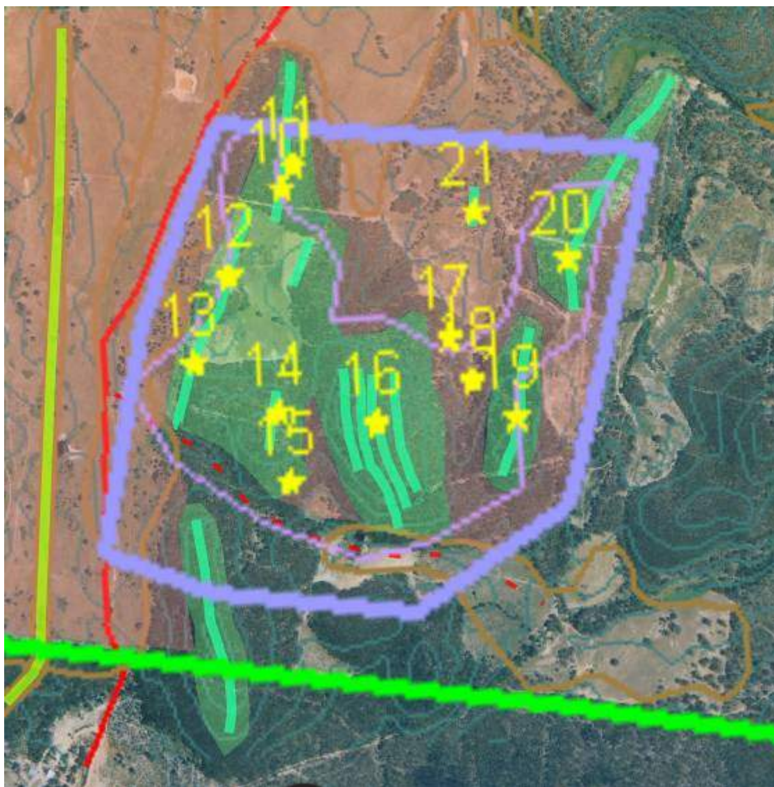
Figure 19 Geological Mapping conducted in the south-east of Marian Vale showing identified areas of hard and soft metasandstone as per the map key.
