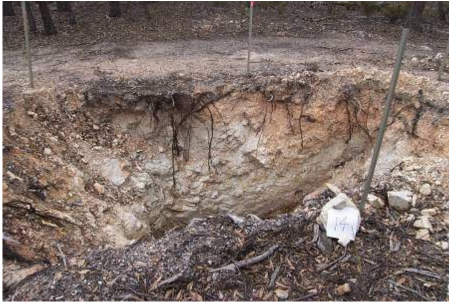
Figure 8 The backhoe pit at site 14 which reveals soft metasilstone that is not evident at the surface.
