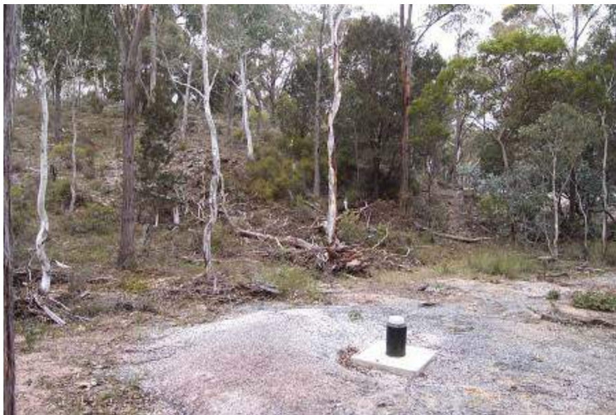
Figure 4 Water bore - site 28. A hard fissured meta-sandstone band is in the background where it forms a spur. Rock chips from the bore give important evidence of the nature and consistency of meta-sandstone/siltstone found in the bore hole along with vein quartz remains.
