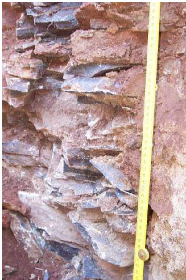
Figure 26. Basalt of a pillar half removed by the backhoe.
