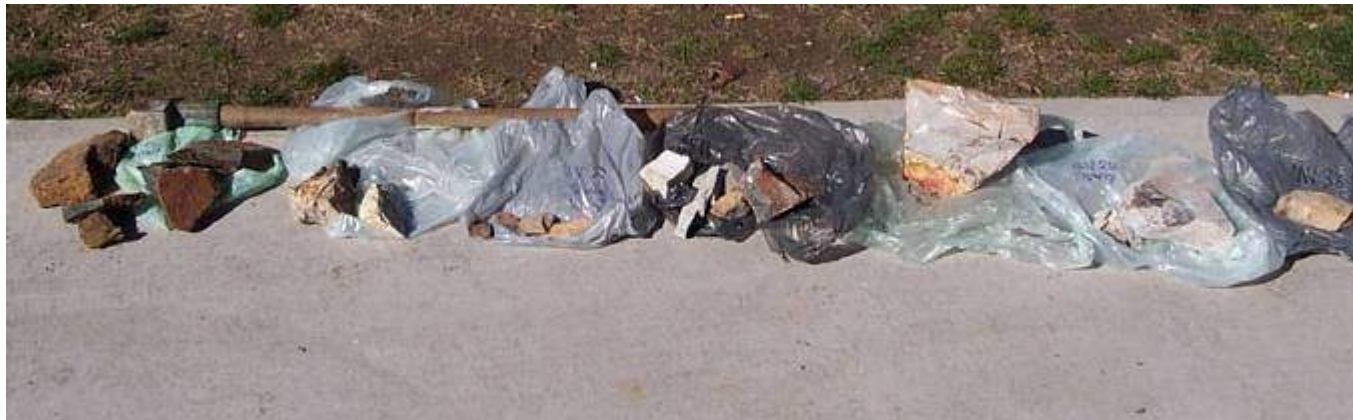
Figure 1 Rock samples from left to right are gabbro (site 36 – backhoe pit), Basalt (site 36 – backhoe pit), quartz vein ridden metasandstone (site ?), Shale flecs (site 30 – western boundary), metasandstone and shale hardened by faulting along with fault plane minerals such as talc (site 32 – bulk sample site), hard metasandstone (site 4 - lookout), Chert and shale (site 25 – quarry), soft metasandstone (site 38).
