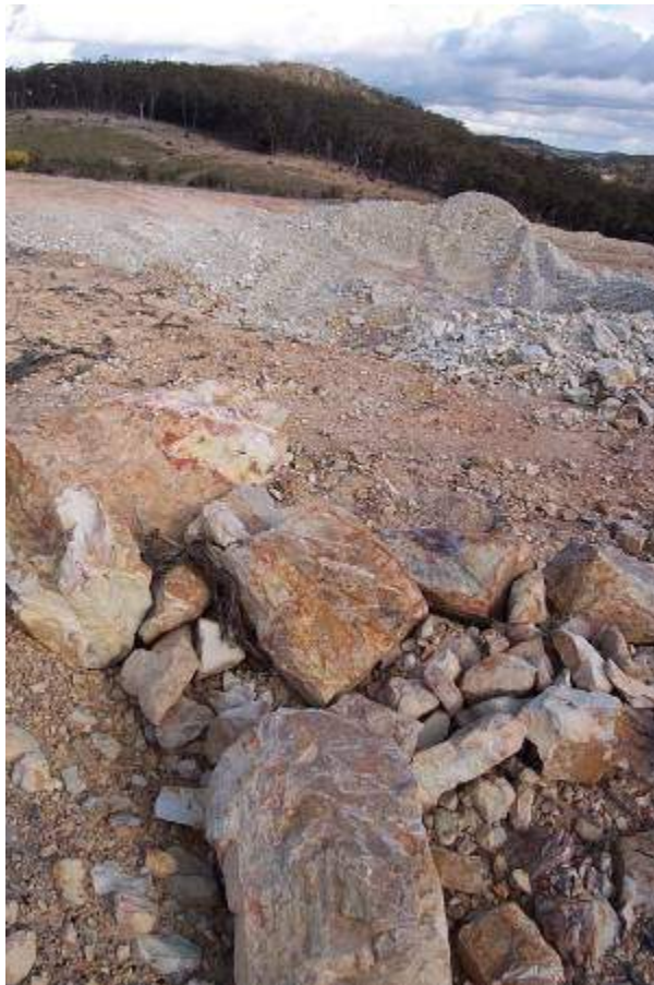
Figure 9 Site 32 Greenish colour on hard blocky metasandstone in the foreground is probably chloritic and is only present around the faults. Highly altered shale (now white) and soft white blocky metasandstone is present in the vicinity of the fault. Greasy minerals including talc, and probably serpentine are on the actual fault plane.
